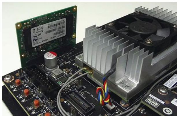
1. Virtium’s StorFly compact SATA SSD with NVidia’s Jetson TX1.
